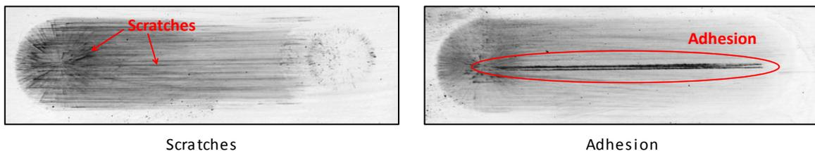
Figure 5: Detection of scratches and adhesion with UV indicators
