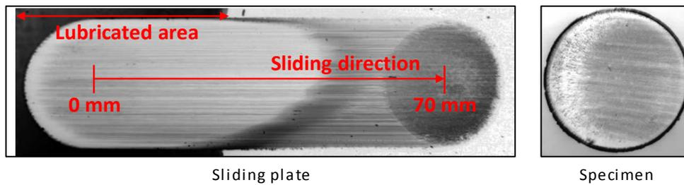
Figure 8: Partly lubricated sliding plate after a Sliding Compression Test
