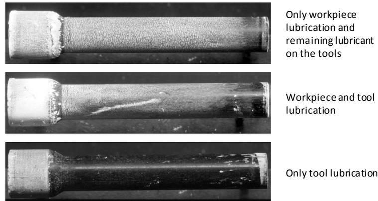
Figure 9: Indirect lubricated specimen of a forward extrusion
