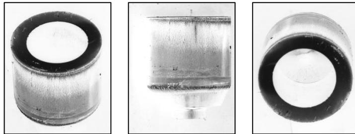
Figure 4: Distribution of the lubricant after the forming process
