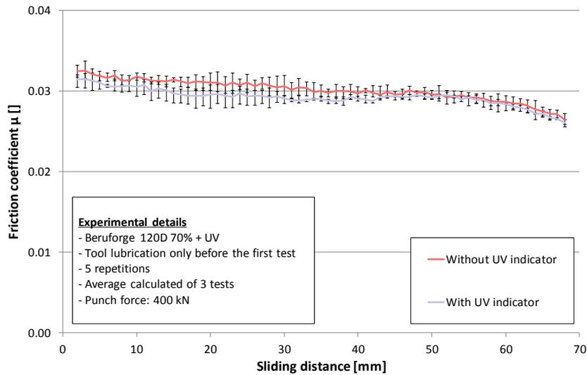
Figure 3: Influence of the UV indicator on the capability of the lubricant
