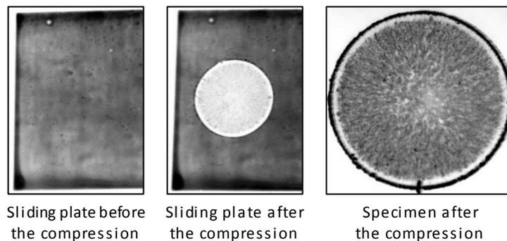
Figure 7: Transfer of the lubricant during the compression
