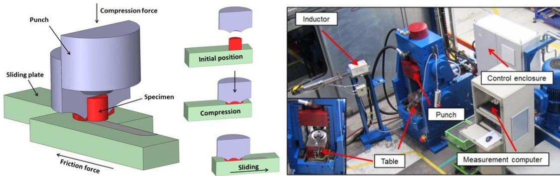
Figure 1: Principal and photo of the Sliding Compression Test [Gro13, Mue13a]
