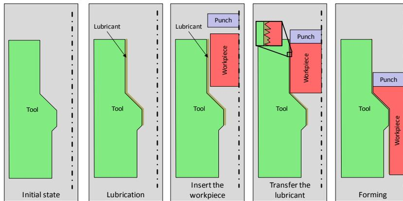
Figure 6: Concept of the indirect lubrication
