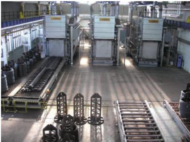
▲ Figure 8. Semi-continuous STC<sup>®</sup>-furnace
