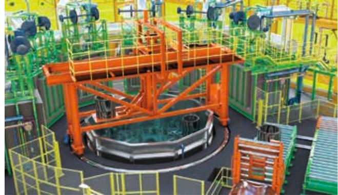
▲ Figure 4. Batch Furnaces incl. quench and manipulators
