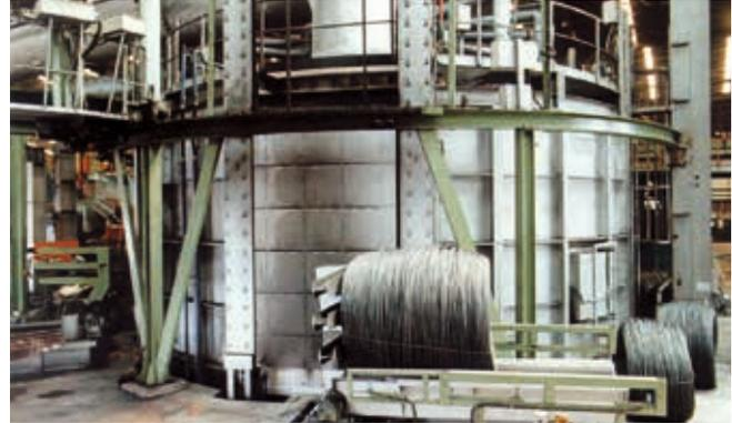
▲ Figure 1. Conti Rotary Table Furnace for solution annealing
