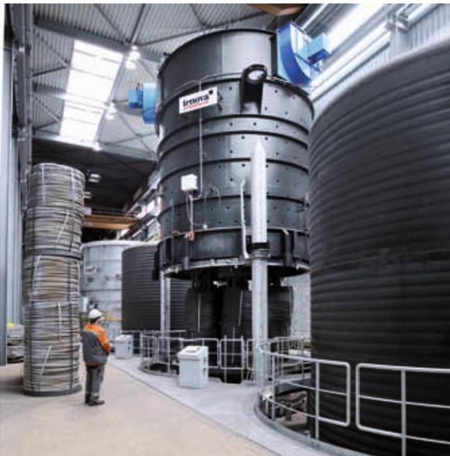
▲ Figure 5. Multi-stack Bell-type Annealing Furnace
