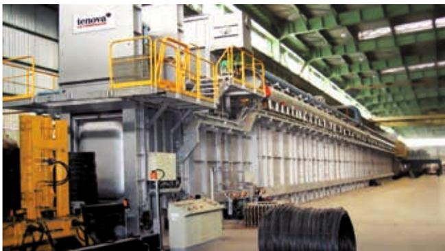
▲ Figure 9. Roller Hearth Furnace for wire coils
