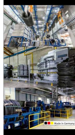
CLAAS/KLINCKE Wireworks are two independent companies that use state-of-the-art drawing machines and the latest annealing and surface technologies to draw and finish wires with diameters from 0.02 to 2.00 inches to a high level of quality.
